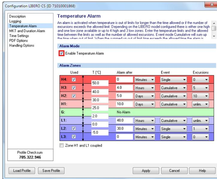
Temperature alarm activated for LIBERO CS and LIBERO CI with multi alarm zones
