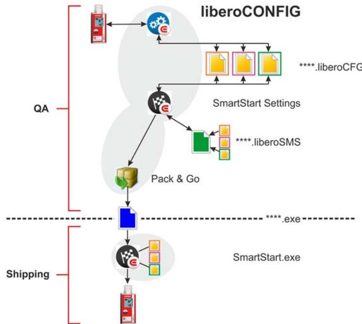
**i** SmartStart Pack & Go exe file with a LIBERO Cx can be used on any PC without installation or a special driver.
